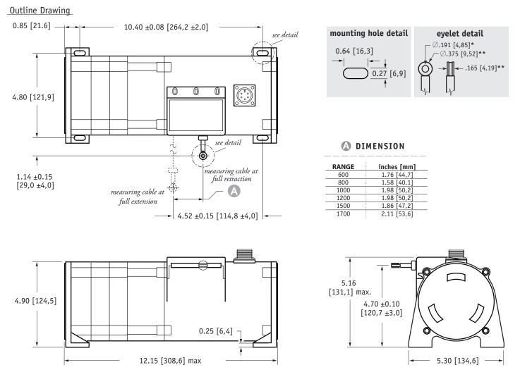
DIMENSIONS ARE IN INCHES [MM] tolerances are 0.03 IN. [0.5 MM] unless otherwise noted.
