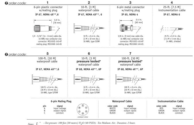
Notes:  $\begin{cases} * & -\text{Test pressure: } 100 \text{ feet } [30 \text{ meters}] H_2 O (40 \text{ PSID}); \text{ Test Medium: Air; Durat} \\ ** & -\text{NEMA 4X applies to stainless steel enclosure only.} \end{cases}$
