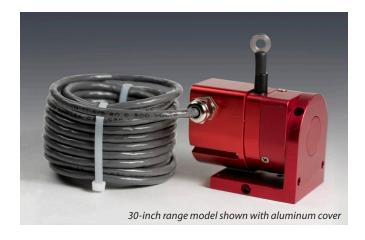
The MT3A is the solution for high-acceleration test applications in potentially wet environments. Just like the MT2A, the MT3A comes in 5 different full-stroke ranges, has a hightension heavy-duty measuring cable designed for the demands of flight and automotive crash tests and comes with an easy to use 2-axis 360° rotation mounting bracket for installation in hard to fit areas.
