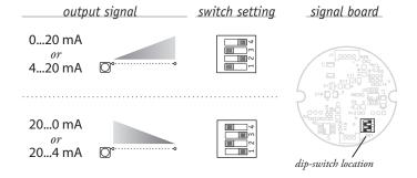
The output signal direction can be reversed at any time by simply changing the dip-switch settings found on the internal signal board. After the settings have been changed, adjustment of the Zero and Span trimpots will be required to precisely match signal values to the beginning and end points of the stroke.
