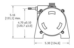
DIMENSIONS ARE IN INCHES [MM] tolerances are 0.03 IN. [0.5 MM] unless otherwise noted. \* tolerance = +.005 -.001 [+.13 -.03] \*\* tolerance = +.005 -.005 [+.13 -.13]
