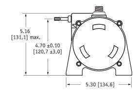
DIMENSIONS ARE IN INCHES [MM] tolerances are 0.03 IN. [0.5 MM] unless otherwise noted.
