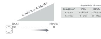
\*note: signal endpoints are set at the time of manufacture and cannot be adjusted
