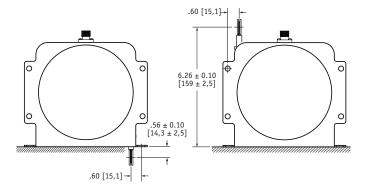
**To change cable exit direction:** simply remove the 4 bracket mounting screws and rotate sensor body to desired direction.
