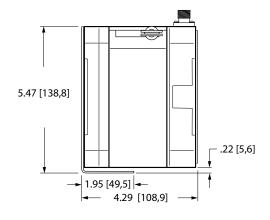
DIMENSIONS ARE IN INCHES [MM] tolerances are 0.04 IN. [1.0 MM] unless otherwise noted.
