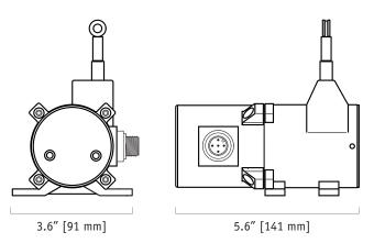
The PT8DN, using a high cycle plastic-hybrid potentiometer, communicates via DeviceNET protocol with programmable controllers in factories and harsh environments requiring linear position measurements in ranges up to 60".
