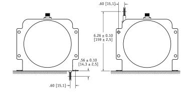
**To change cable exit direction:** simply remove the 4 bracket mounting screws and rotate sensor body to desired direction.
