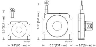
A perfect solution for both OEM and single-piece user, this string pot provides an economically priced CANopen sensor for 80-inch and 120-inch stroke range applications. This sensor is constructed with a rugged polycarbonate enclosure, a stainless steel mounting bracket and universally accepted M12 connector for operation in both outdoor or factory dry environments. For the OEM, customized options are available.
