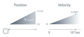
\*velocity output rate =  $361 \text{ mV} \pm 3\%$  @ 100 inches per min.
