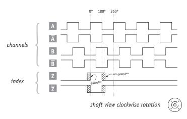
\*\*note: - 1000, 2000, 2500 pulses-per-turn options — gated to A , index pulse = 180° - 100 pulses-per-turn option — ungated, index pulse = approx 270°
