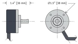
The CS15 is Celesco's compact industry standard size 15, servo-mount incremental encoder. With a low profile of less than an inch in height and a diameter of only 1.5 inches, the economically priced CS15 is perfect for both the OEM and single-piece user alike. Precision ball bearings support a durable stainless steel shaft for reliable, long life operation.
