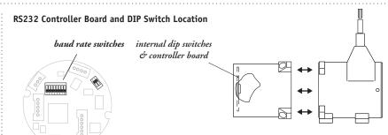
to gain access to the controller board, remove four Allen-Head Screws and remove rear cover.
