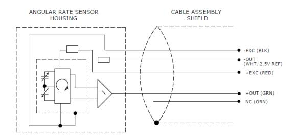
SHUNT CALIBRATION SUPPORTED FOR EITHER OUTPUT LEAD TO BLACK LEAD. UNIT BEHAVES LIKE 400 $\Omega$  BRIDGE POWERED BY 5V EXCITATION.
