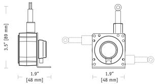
The Celesco SE1 is the digital encoder version of our compact String Pot series. The SE1 is an economical and durable device that utilizes a flexible cable, a spring-loaded spool and an incremental optical encoder to detect and measure linear position.
