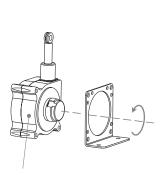
For added flexibilty, mounting bracket can easily be switched to the opposite side.
