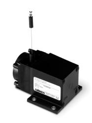
The PT1232, part of our compact line of cable extension transducers, delivers position feedback via RS232 serial communication to your data acquisition or controller system. The PT1232 sends a raw 16-bit position count from 0000 to FFFF (hex). Additionally this device can be set to continuously send data or send data only when polled.
